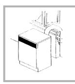
The end of the tube should be directed downwards, to prevent warm moist air from condensing in the room or in the dryer.
